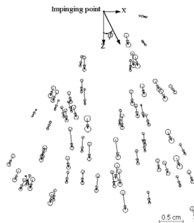
Fig. 12. PIV results for the asymmetric impinging jets for m_w:m_s = 2:1 , \theta = 90^\circ .
